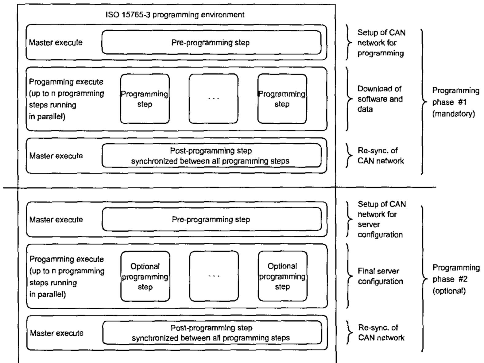
Figure 20 — ISO 15765-3 non-volatile server memory programming process overview
