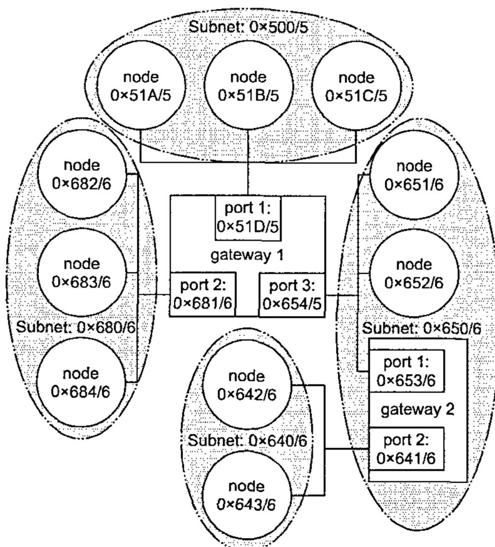
Figure 13 — Network configuration example
