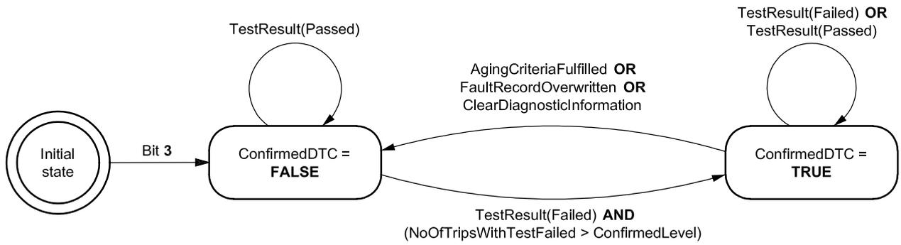
Figure D.4 — DTC status bit 3 confirmedDTC logic
