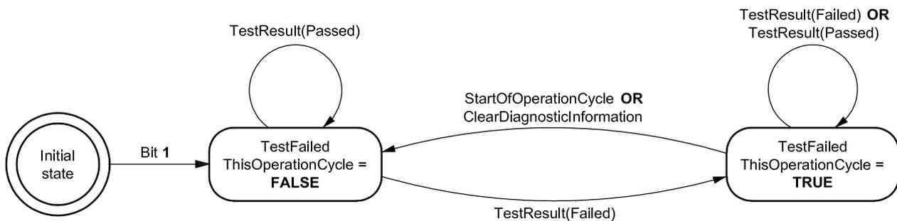
Figure D.2 — DTC status bit 1 testFailedThisOperationCycle logic
