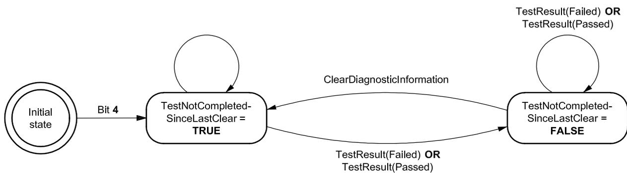
Figure D.5 — DTC status bit 4 testNotCompletedSinceLastClear logic
