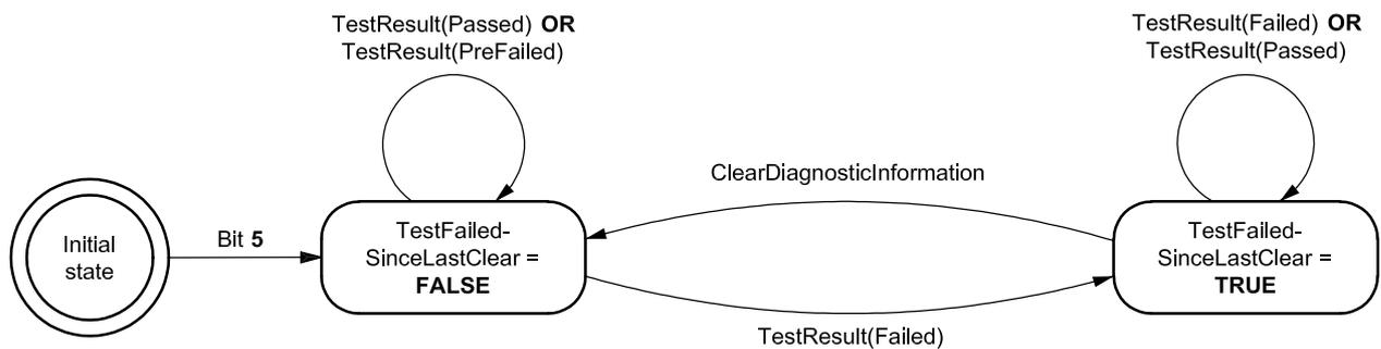
Figure D.6 — DTC status bit 5 testFailedSinceLastClear logic
