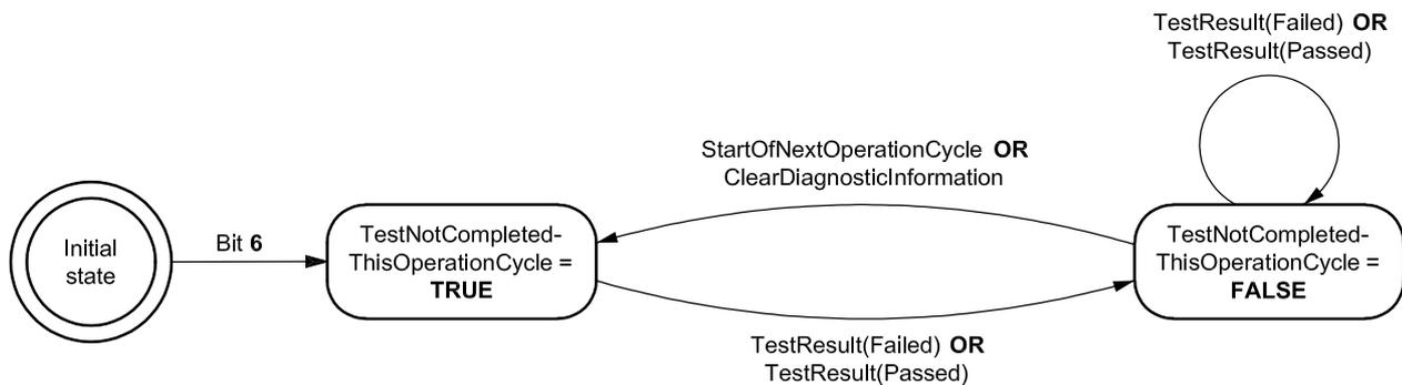
**Figure D.7 — DTC status bit 6 testNotCompletedThisOperationCycle logic**
