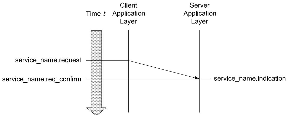
Figure 5 — Application layer service primitives — unconfirmed service
