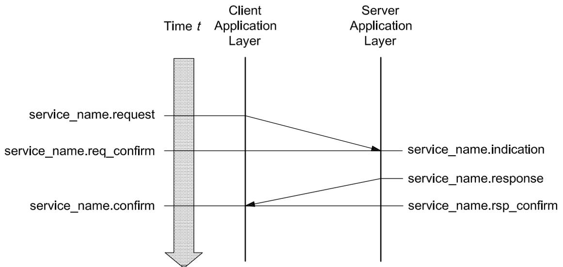
Figure 4 — Application layer service primitives — confirmed service
