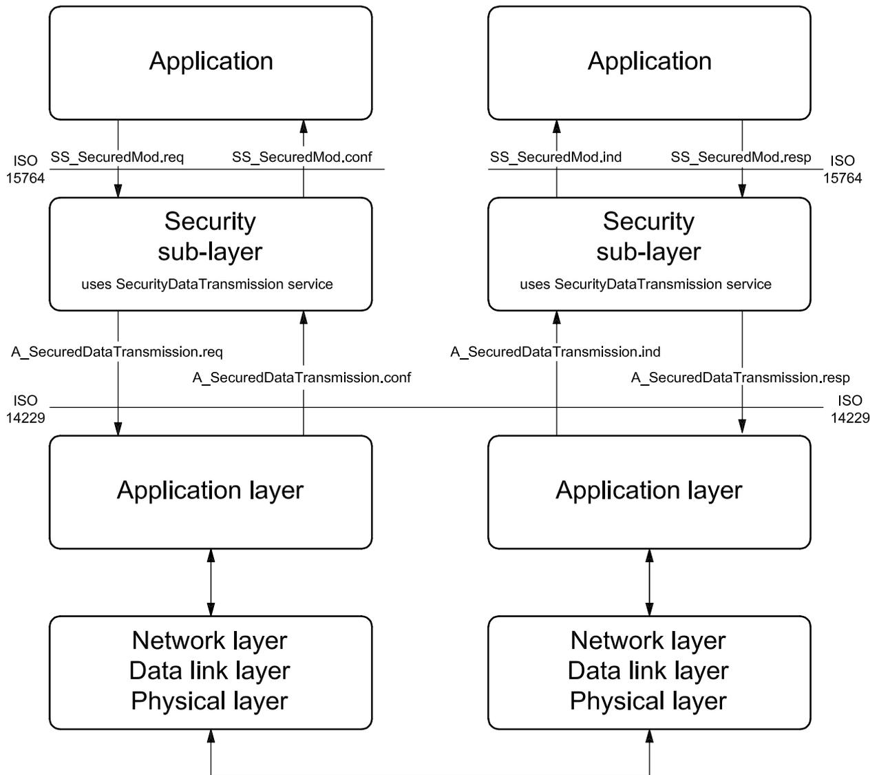
Figure 11 — Security sub-layer, application layer and application interaction
