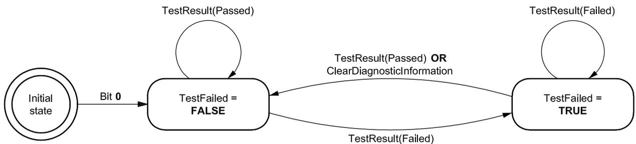
Figure D.1 — DTC status bit 0 testFailed logic
