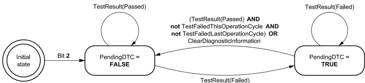
Figure D.3 — DTC status bit 2 pendingDTC logic
