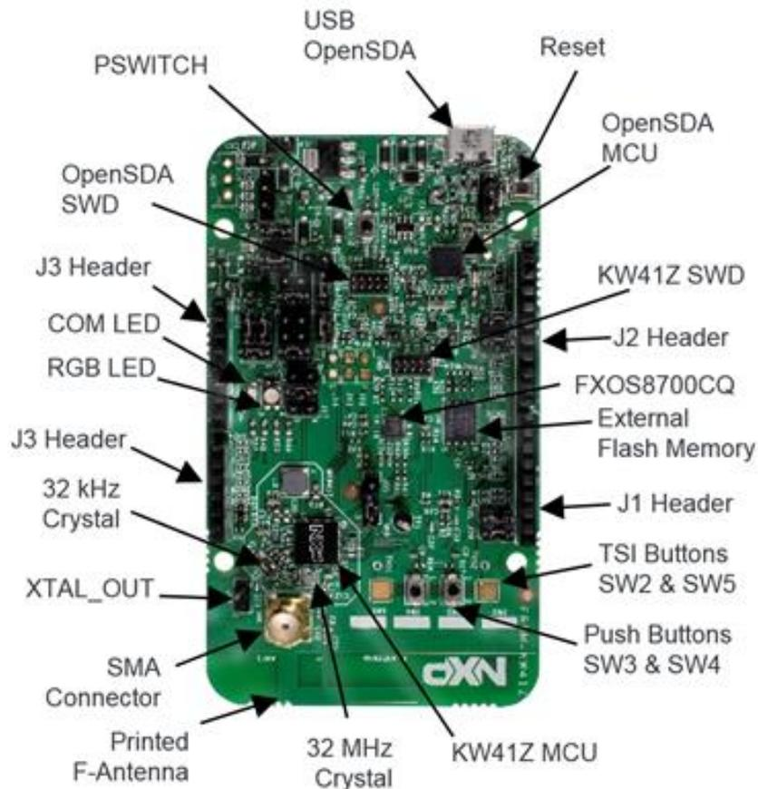
Figure 3: FRDM-KW41Z component placement.
