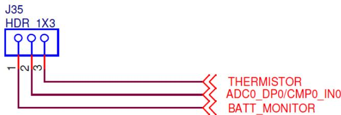
Figure 16: ADC0\_DP0 selection jumper.
