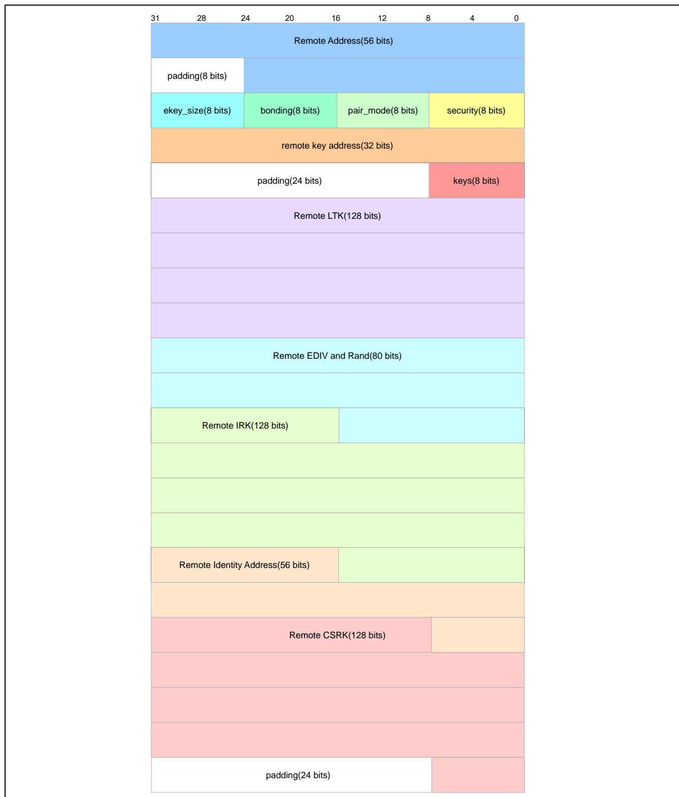
Figure 5.10. Remote device security data structure
