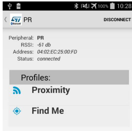
In this case, two services are exposed: **[Find Me]** (see Section 2.4.6.7 Reading FMT Data on smartphone) and **[Proximity]**. After the latter, you can set the alert level to be generated remotely in case of disconnection or link loss. You can also set the path loss threshold: if the path loss exceeds a certain level, an alert signal is remotely generated.
