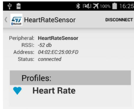
To obtain heart rate measurements, select **[Heart Rate]** service. The following figure shows heart rate characteristics obtained from the heart rate sensor. You can read the real-time heart rate value, the sensor location and the graph displaying the latest heart rate values.
