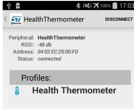
To obtain temperature measurements, you should select [Health Thermometer] service. The following figure shows health thermometer characteristics being obtained from the HTM sensor. You can read the real-time temperature value and the graph displaying the latest temperature values.
