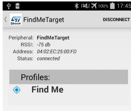
After selecting the [Find Me] service, you can generate an alert signal on the remote device by pressing the related button as shown below.
