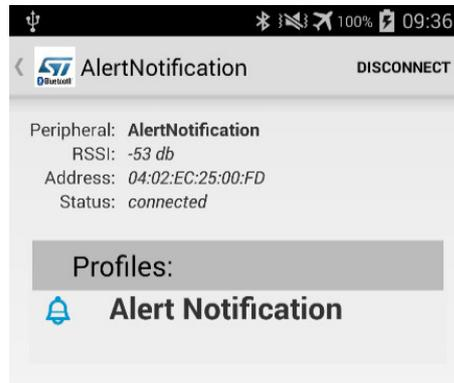
To perform actions on the ANS device, select the [Alert Notification] service. The following figure shows the list of alert categories provided by the ANS, the alert details and the selectable options for notifications about a specific set of alert categories. In this case, the ANS provides the Email alert category.
